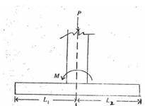
A rectangular reinforced concrete footing is to be designed to support a column which transfers axial load and uniaxial moment to the footing as shown in the above figure. The footing is to be designed to have uniform upward soil pressure. The dimensions  $L_1$  and  $L_2$  ( $L = L_1 + L_2$ ) of the footing would be
