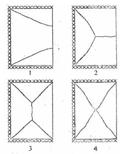
A reinforced concrete rectangular slab is built-in (fixed) on three edges and the other edge is free. The possible yield line patterns for the slab subjected to a uniformly distributed load and reinforced isotropically are shown above as 1, 2, 3 and 4.
