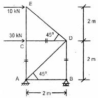
A pin jointed truss is loaded as shown in the above figure match List I with list II and select the correct answer:
